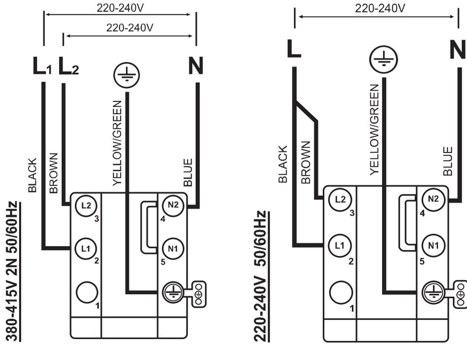
The induction hob is composed of 2 modules, each one can absorb 3.7kW max.
